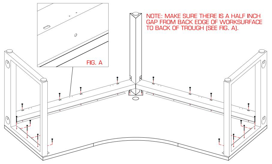
6. IF SCREENS WHERE ORDERED WITH STATION, ATTACH SCREEN BRACKETS TO TROUGH AS SHOWN BELOW USING HARDWARE PROVIDED.
